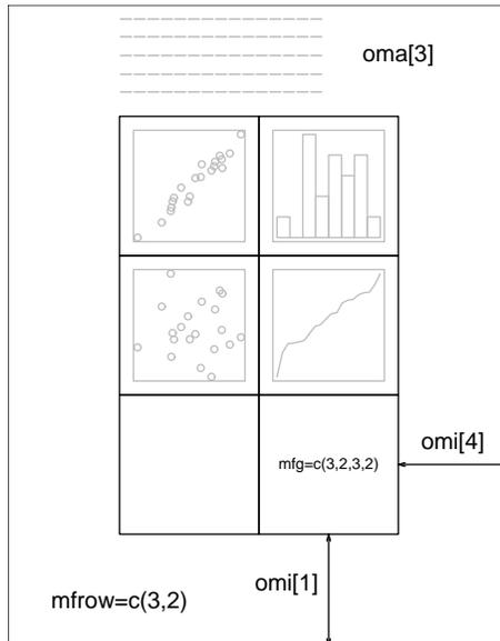
**oma** A vector of the form  $c(x1, x2, y1, y2)$  giving the region *inside* outer margins in NDC (= normalized device coordinates), i.e., as a fraction (in  $[0, 1]$ ) of the device region.
