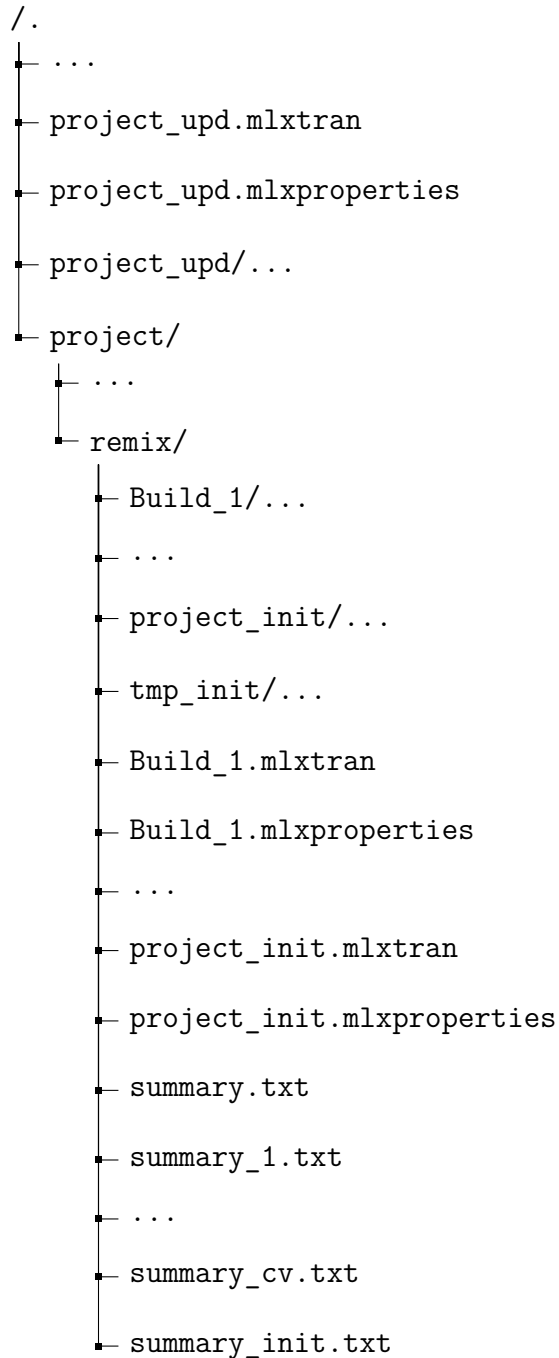
Figure 10: Structure of a Monolix project directory after sequential execution of initStrat , remix , and cv.remix , with both unlinkTemporaryProject and unlinkBuildProject set to FALSE . The remix folder contains all temporary projects and summary files generated during initialization, cross-validation, and final estimation steps.
